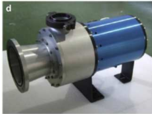
Figure 5: A photograph of the R245fa turbogenerator [7].
