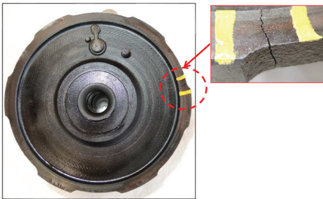
Figure 2. Breakage of the flange of bearing housing.
