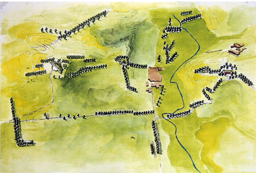
Fig. 4. A system of the “masks” – the artificial groves and greenbelts, fulfilled a function of a giant dark screen, covering silhouettes of the forts and batteries on the skyline, visible from presumed enemies positions. The 6 th Fortified Sector of the Fortress (reconstruction – J. Środulska-Wielgus)
