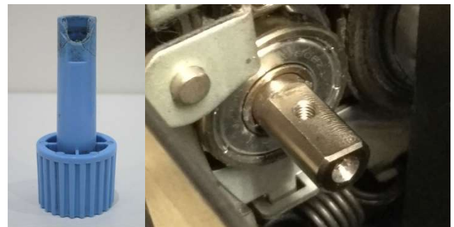
Fig. 3. Knob that mates with the fusing heating unit: a) knob defective, b) mating element
