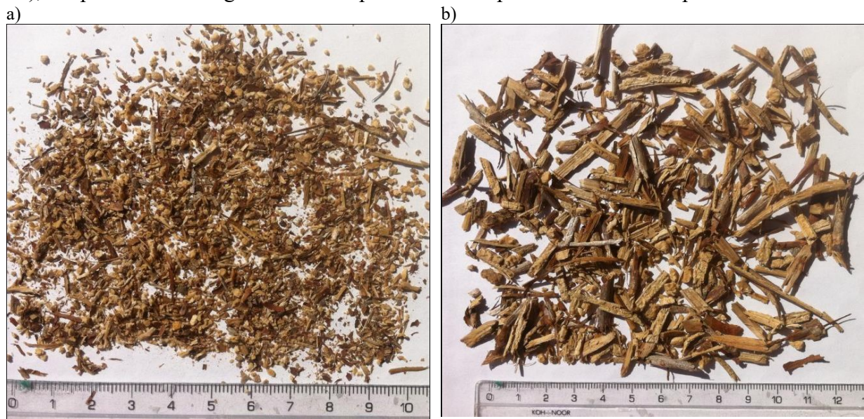
Figure 1. The pictures of raspberry particles used in research to produce face (a) and core (b) layers of particleboards (source: own research)
