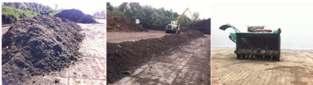
Photo 1. Composting of waste in prisms, from the left prism after transferring the first day of research, prism on the last day of the intensive composting process, mobile turning machine.
