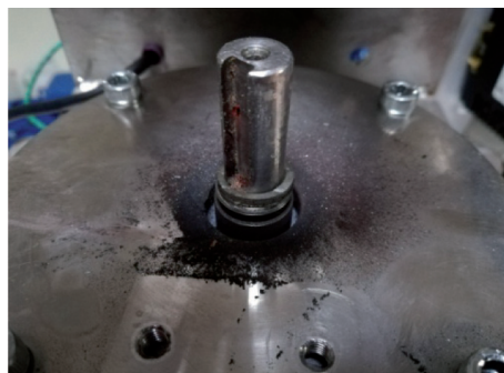
Fig. 7. View of the accumulated metal filings on the upper part of the clutch body
