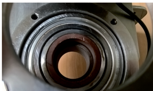
Fig. 8. View of the textolite burn at the bearing seat
