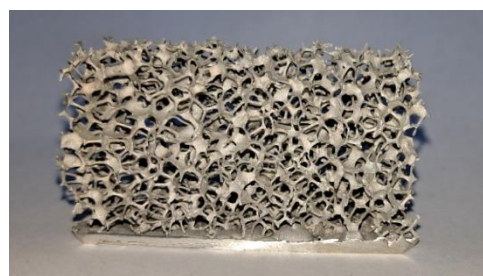
Fig. 2. AZ91 magnesium alloy sample (55x35x20 mm) produced from 20 PPI polyurethane foam
