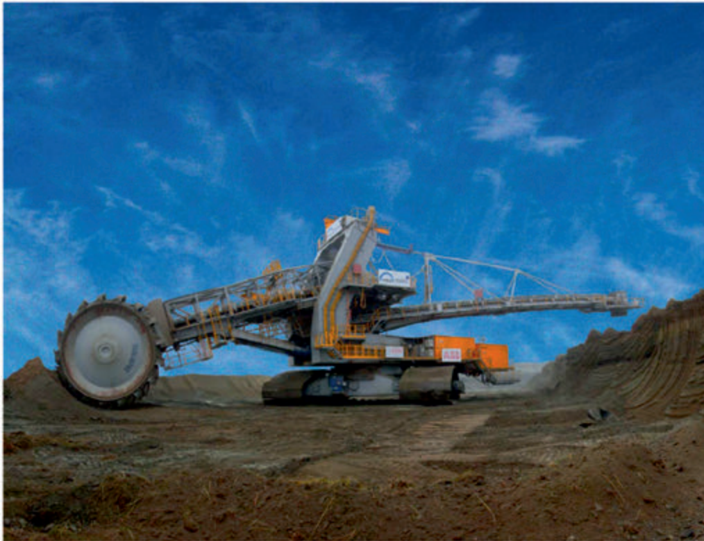
Rys. 4 Kompaktowa koparka SRs(H) 1050.23/2.0 [7] Fig. 4. Compact bucket wheel excavator SRs(H) 1050.23/2.0 [7]
