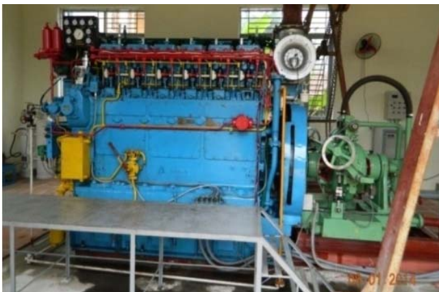
Figure 6. The marine diesel engine Yanmar 6S185L-ST
