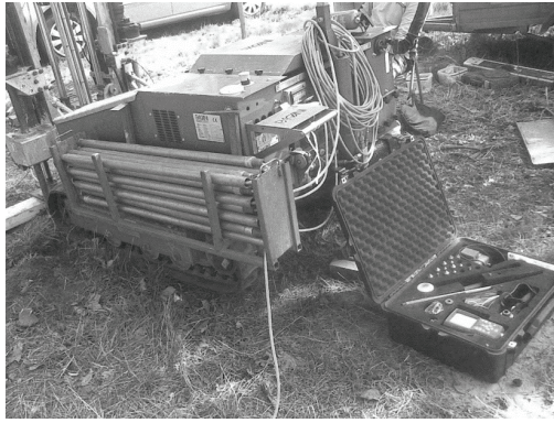
Fig. 2. CPTU test rig and Panda 2 prepared for testing
