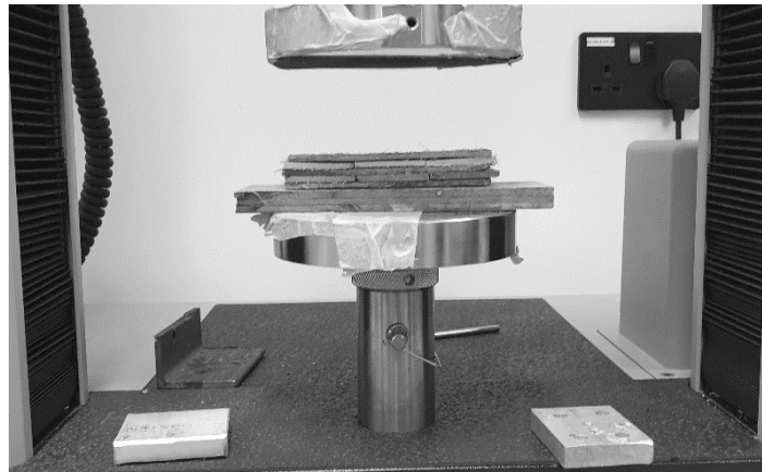
Fig. 2. Applying clamping pressure on a 5 layer specimen using a UTM
