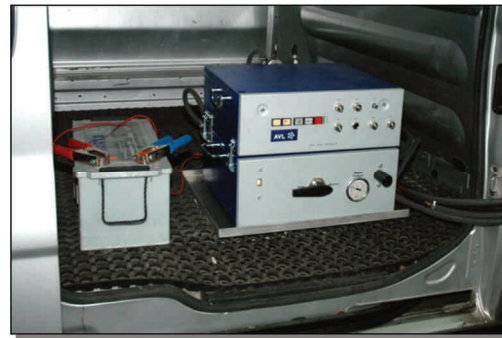
Fig. 4. KMA Mobile Fuel Flow Meter
