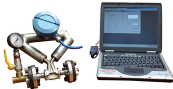
Fig. 5. CMF 025M Mass Flow Meter From Emerson
