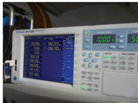
Fig. 6. Yokogawa WT 1800E Power Analyzer
