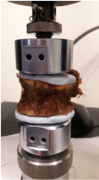
Fig. 2. Lumbar vertebra before failure. The resin is placed at the top and the bottom of the vertebral body
