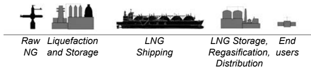
Figure 2. LNG supply chain (the authors' elaboration based on (Mokhatab, et al., 2014))
