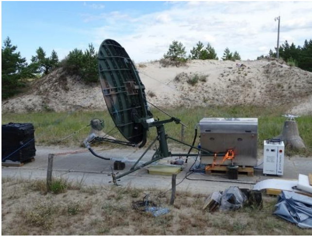
Fig. 4. HPM antenna and generator
