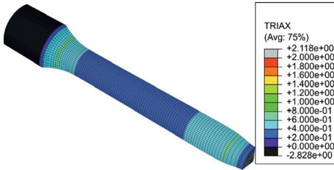
Fig. 7. Distribution of the parameter \eta during the formation of the plastic neck
