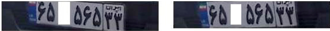
Fig. 10. (a) extract, (b) Rotate correction of a sample ROI (in order to comply with privacy, part of the plate has been hidden)
