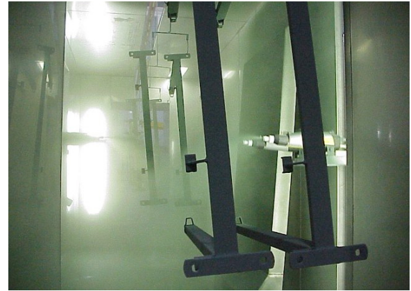
Figure 5 Paint booth for automatic powder paint application
