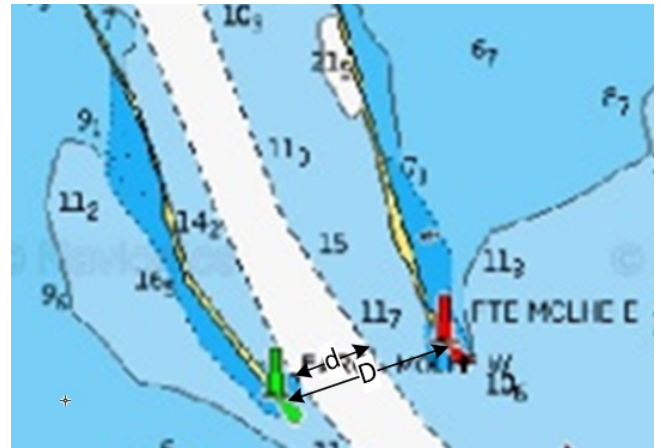
Figure 2. The method of sizing of the entrance to the port.
