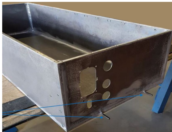
Fig. 11. A case for a 600V battery system of the electric vehicles
