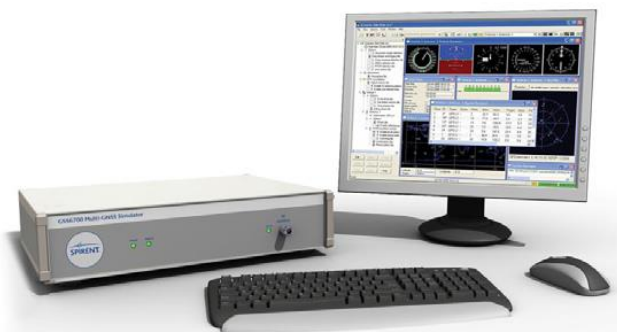
Fig. 5. The Spoofer – complex computer and radio equipment for the implementation of GNSS spoofing. It costs several thousand dollars. The source SPIRENT https://www.spirent.com
