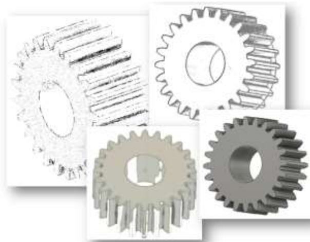
Fig. 7 3D scanning of the reconstructed object
