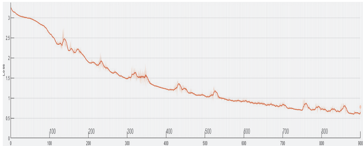
Figure 15. Fixing 1 volume hour learning loss chart using the Adam method. Y axis - losses, X axis at the top - number of epochs (max 900), X axis at the bottom - number of iterations (max 900). Source: own study [2, 15].
