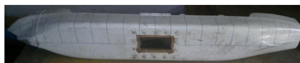
Fig. 4. Bottom view of ship model with moonpool
