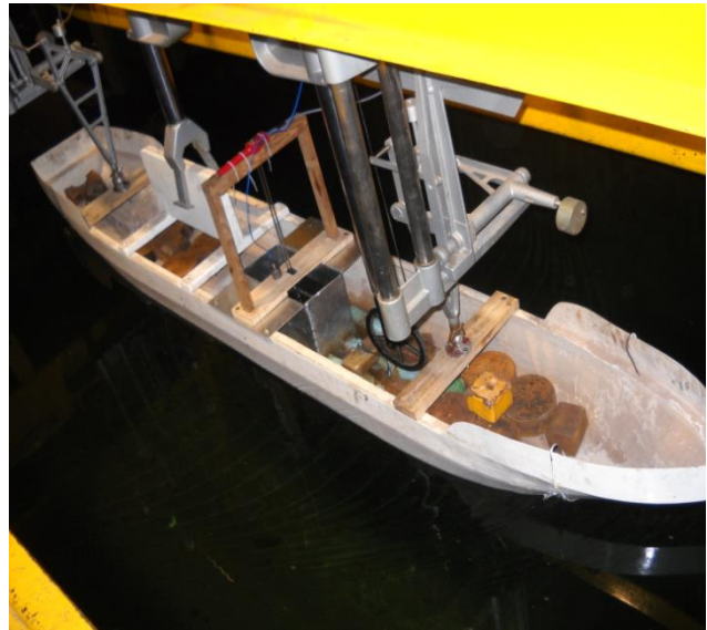
Fig. 6. Model in towing tank with forward speed
