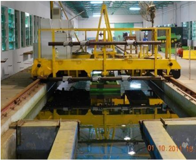
Fig. 5. Towing tank at Dept. of Ocean Engg., IIT Madras.
