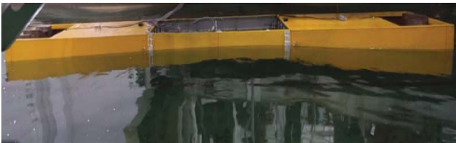
Fig. 6. Collapse test of ship hull
