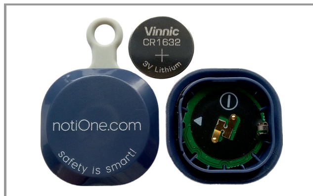
Fig. 4. Opened notiOne beacon with a CR1632 button cell battery.
