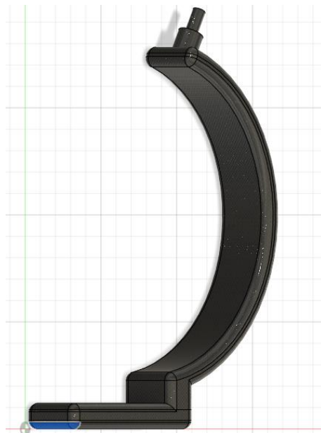
Figure 2. The model of foot prosthesis fixed on the curved surface of the bottom layer of the base (this curved surface is marked on blue).
