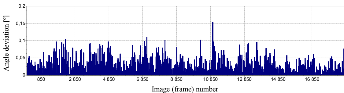
Figure 5. Graph of the absolute difference between the angles derived from the video image and as measured by inclinometer (1 image estimate per second)
