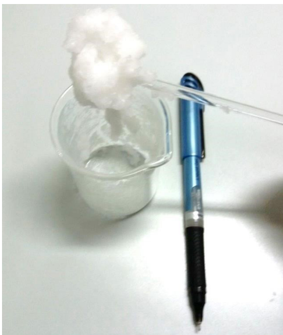
Figure 2. Gel explosive (HPOM type) formed from highly concentrated hydrogen peroxide and polymer organic fuel [source: authors]
