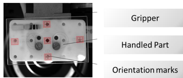
Fig. 7. Acquired image of the bottom camera. Measuring the real movement of the robot
