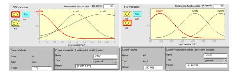
Fig. 4. Membership function of fuzzy sets for input variables
