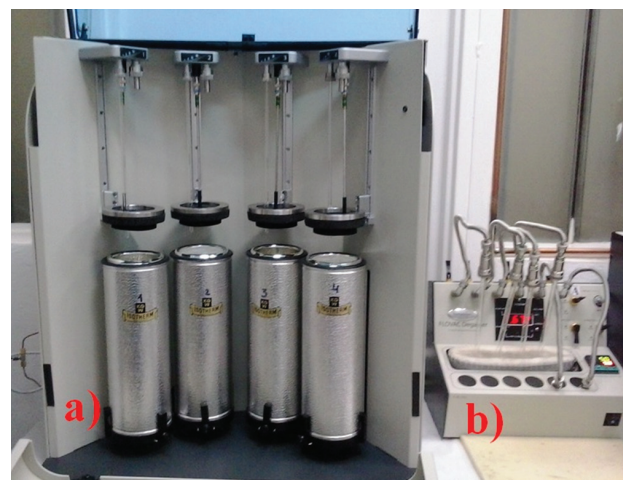
Fig. 1. An apparatus for the measurement of specific surface area (a) and a sample degassing station (b).
