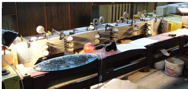
Fig. 3. Test stand with eccentrically compressed RC column
