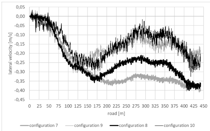
Fig. 9. Lateral velocity on a dry and an icy, randomly uneven road surface with the almost different left and right profiles of irregularities ( cor_H = 0.2 ) [own research]
