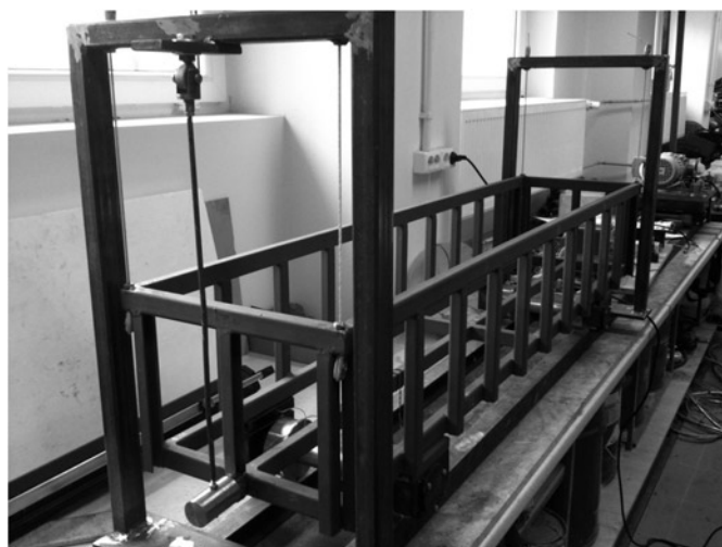
Fig. 4. Model of the freight car (the half-determined system) together with the pendulum
