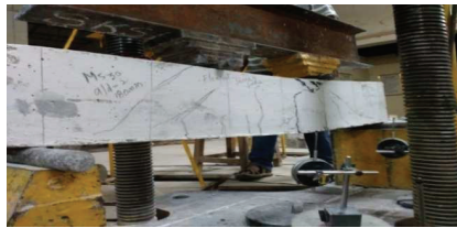
Figure 11 Failure pattern of SFSCC30
