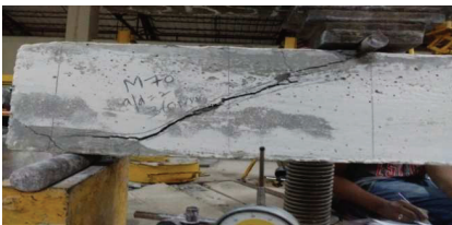
Figure 12: Failure pattern of SCC70
