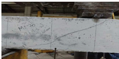
Figure 13: Failure pattern of SFSCC70
