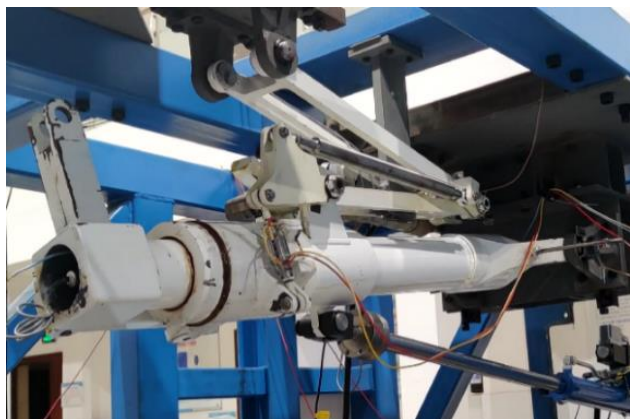
Fig. 6. Retraction mechanism experimental prototype.
