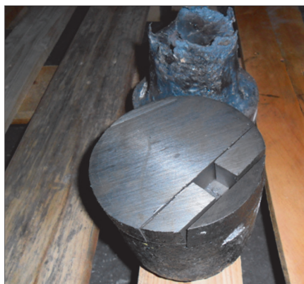
Fig. 10. Cast ingots and the sampling location for microscopic studies of morphology of non-metallic inclusions
