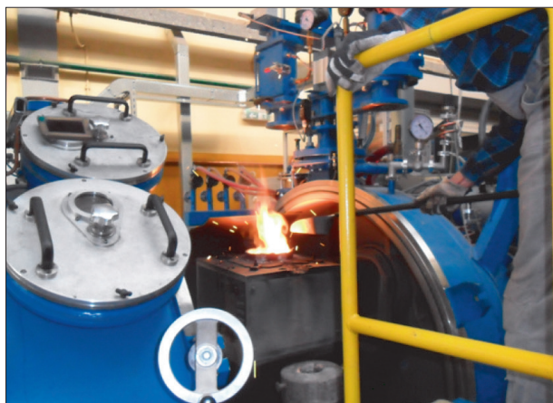
Fig. 7. Adding composite pellets in portions into liquid steel
