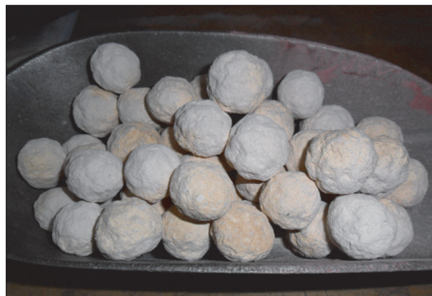
Fig. 5. Portion of PLAS10 pellets prior to dropping into a metal bath
