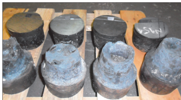
Fig. 9. Cast ingots from four laboratory heats
