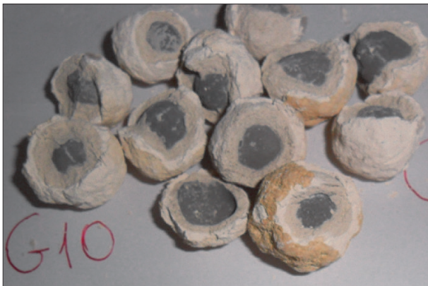
Fig. 6. Composite pellets after a drop test: a) P 25 pellets, b) Al Ca SLAG 70 pellets, c) P 10 pellets, d) LASS pellets
