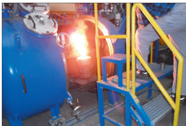
Fig. 8. Casting liquid steel into the casting mould
