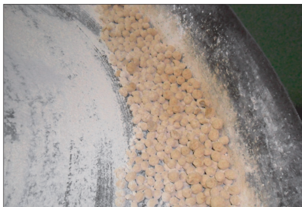
Fig. 4. Pellets on a balling disc during the process of applying the outer layer
