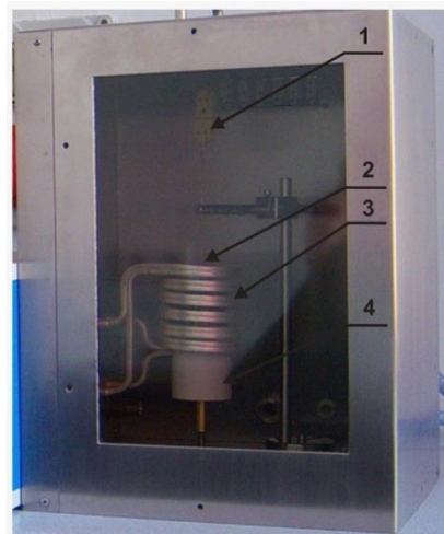
Fig. 1. a) Graphite crucible, b) Working chamber of the UMMA device: 1 –thermocouple, 2 – tested sample, 3 – induction coli, 4 – ceramic isolation
