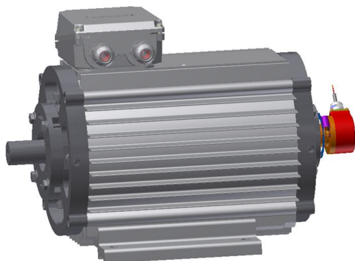
Fig. 2. 3D Motor model with adjustable discs which allow for the regulation of the gap
