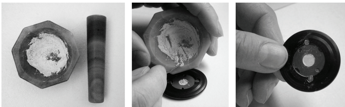
Fig. 2. Sample preparation for X-ray powder diffraction; fine powdered ashed bone respective Brushite (left); the placed samples between two plastic tapes in the sample holder (middle and right)
