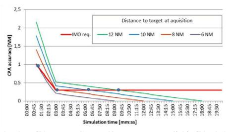
Figure 5. Calculated maximum CPA errors according to tracking target accuracy specified for CPA and relative course – Scenario 2\_1 (relative speed: 40.0 kn)
