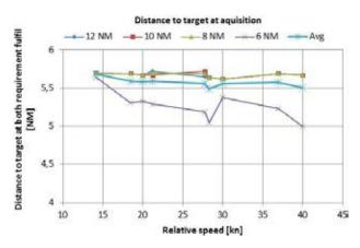
Figure 7. Distance to target when both IMO requirements are fulfilled
