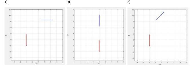
Figure 2. Examples of simulated scenario types: a) Scenario 1\_2, acquisition range – 12 NM, b) Scenario 2\_2, acquisition range – 12 NM, c) Scenario 3\_2, acquisition range – 12 NM (red vector – OS course and speed, blue vector – TRGT data)
