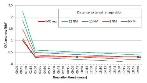
Figure 4. Calculated maximum CPA errors according to tracking target accuracy specified for CPA and relative course – Scenario 1\_3 (relative speed: 14.14 kn)
