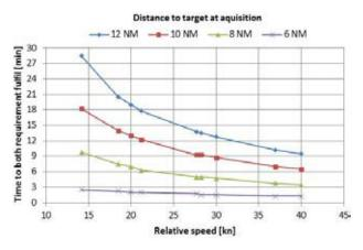
Figure 6. Tracking time when both IMO requirements are fulfilled
