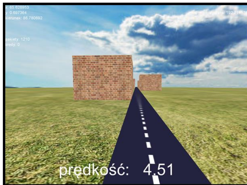
Fig. 2. Simulation of wheelchairs ride generated and displayed in real time by the mechatronic simulator. Legend: „prędkość” – wheelchairs velocity [km/h]; „dystans” – travelled distance [m]; „kierunek” – riding direction [°]
