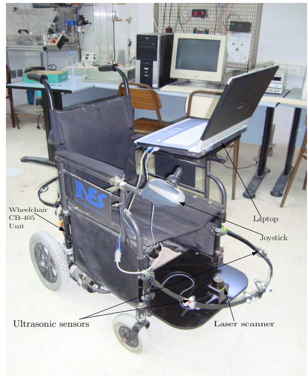
Fig. 1. "Current configuration of the wheelchair. The software on the Laptop uses the measures from the CB405 and the laser to control the wheelchair motion" [2].
