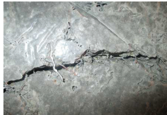
Fig. 12. The Development of Cracks around Steel Fibre.
