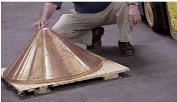
Fig. 9. Outside view of extremely large shaped charge liner used in Russian cruise missiles [32].
