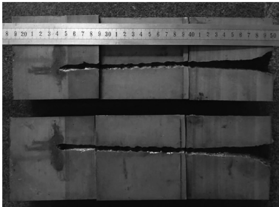
Fig. 8. Experiments on standard shaped charge. For general research, the 56 mm standard shaped charge is adopted. The jet tip velocity is 6453 m/s, and that of the tail is 1179 m/s. The length of the jet at 80 mm standoff equals 111.5 mm [31].
