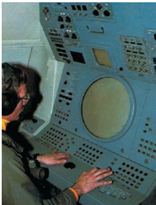
Fig. 16. TACCO & Track Ball (early mouse)
