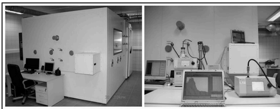
Fig. 3. From left: radon chamber; SMPS and APS particle spectrometers (TSI, USA).
