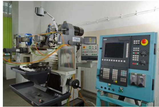
Fig. 3. Machining to create spherical elements from ceramic materials – the system was built based on the milling FNX 30P with Siemens system control [16].
